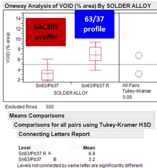
**Figure 14.** Voiding for the Sn63/Pb37 solder paste and the 20-mil stencil web, comparing the SAC305 profile and Sn63/Pb37 profile. The Sn63/Pb37 profile is denoted by an “R” after the alloy.
