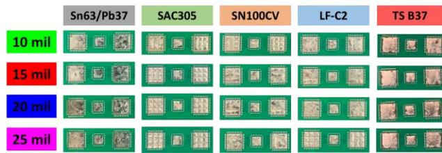
**Figure 8.** Solder spread in the QFN thermal pads for each solder alloy and gap size.
