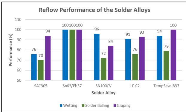
**Figure 7.** Wetting, solder balling, and graping performance for each solder alloy using the SAC305 reflow profile.
