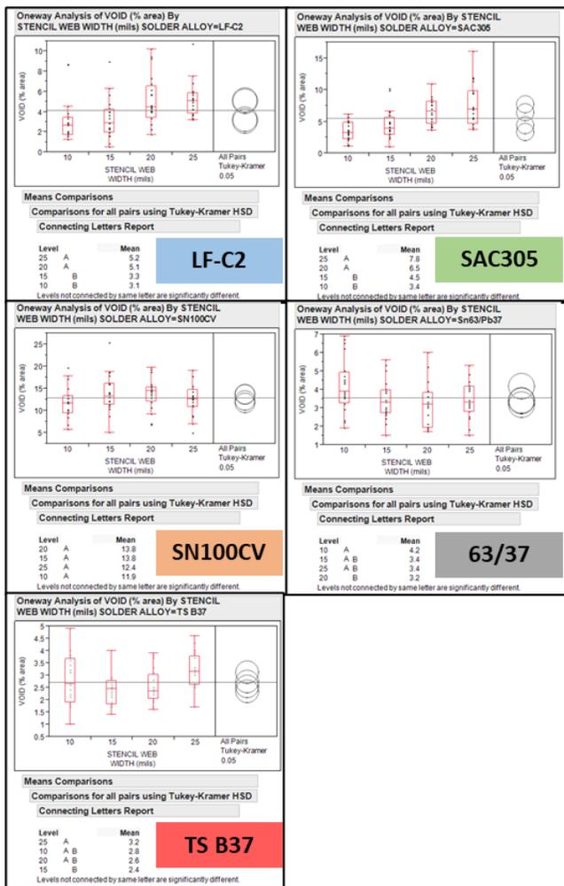
**Figure 13.** Statistical analysis of voiding by solder alloy broken out by web width.
