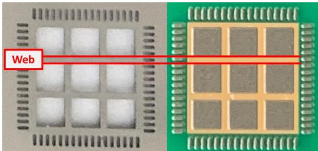
**Figure 2.** Web gaps in the stencil and solder paste print.
