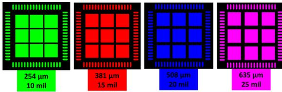
**Figure 4.** QFN68 Stencil Designs in the Thermal pads.
