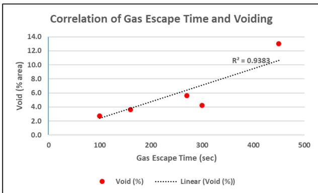
**Figure 10.** Correlation of gas escape time to voiding.
