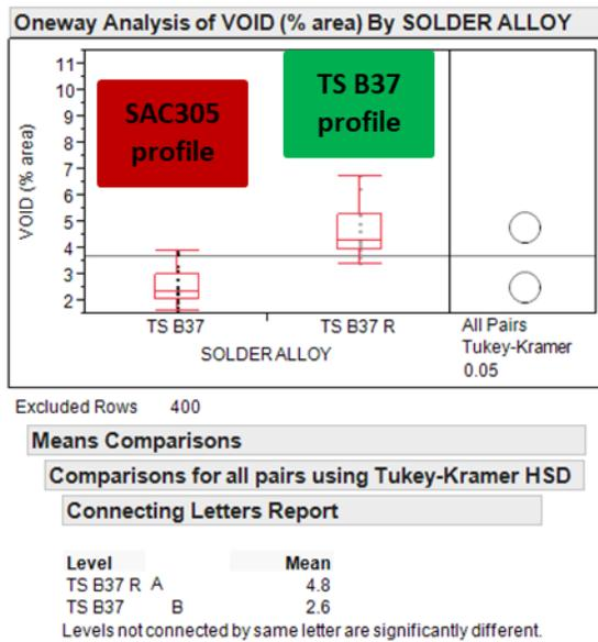
**Figure 15.** Voiding for the TempSave B37 solder paste and the 20-mil stencil web, comparing the SAC305 profile and TempSave B37 profile which is marked with an “R”.
