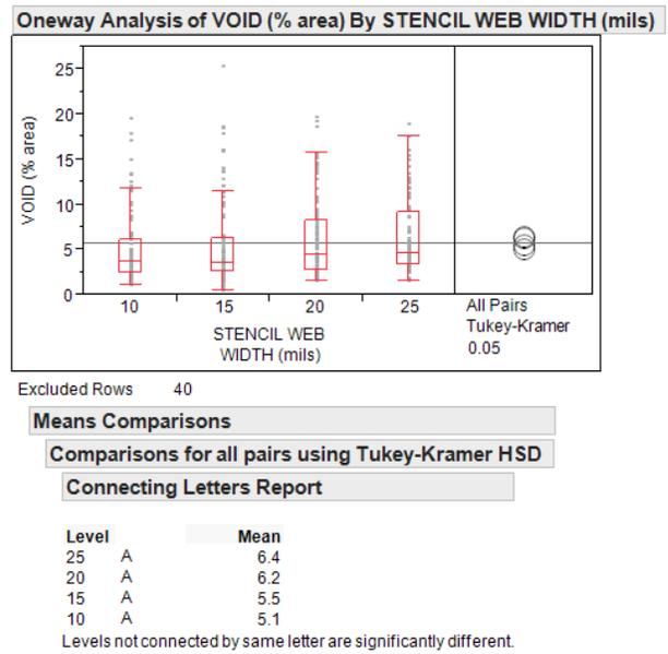
**Figure 11.** Voiding by stencil web width including all solder alloys.
