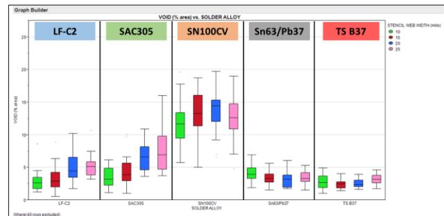
**Figure 12.** Voiding by solder alloy broken out by web width. Green = 10 mil, Red = 15 mil, Blue = 20 mil, and Pink = 25 mil.
