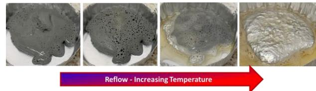
**Figure 6.** Solder Paste Melting and Gas Entrapment
