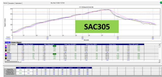
**Figure 5.** Linear RTS Reflow profile for SAC305.
