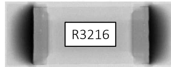
X-ray image after soldering
