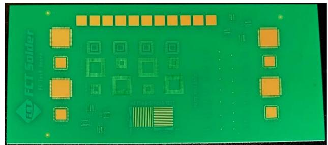
**Figure 5.** PR test board v2 from FCT Solder.
