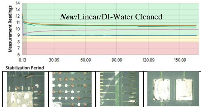
**Figure 19:** *New* Solder Paste/Linear/DI-Water Cleaned
