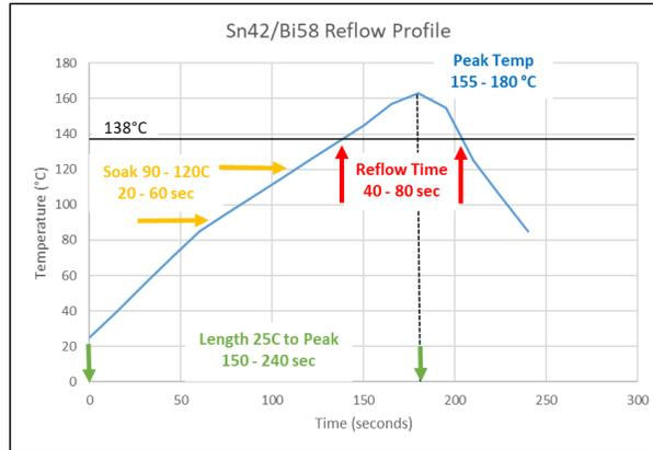
Sn/Bi alloys should not be mixed with lead (Pb) bearing metals. If Pb is mixed with Sn and Bi, then a very low melting (approx. 95 °C) intermetallic compound can form. This very low melting Sn/Bi/Pb compound may cause solder joint failure due to heating during operation of the electronics.
