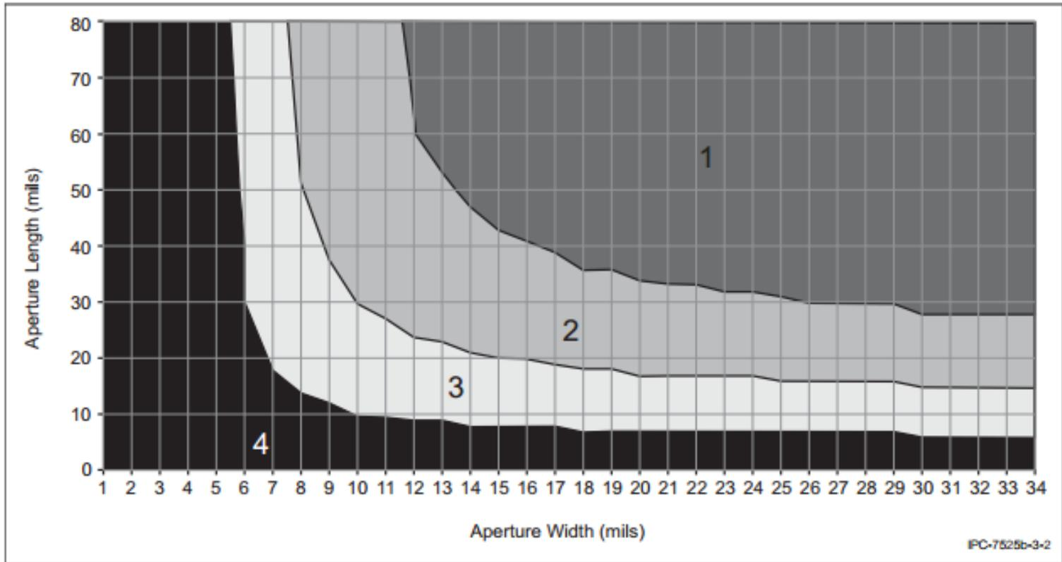
Figure 3-2 5 mil Thick Stencil Tin Lead and Lead Free
